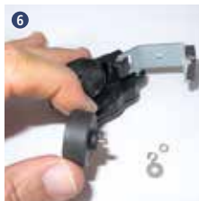
Diaphragm is removed from the magnet bracket
