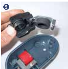
Diaphragm including the magnet bracket is pushed to the outside by pressing against the rubber insert
