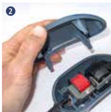
Pump cover is removed
