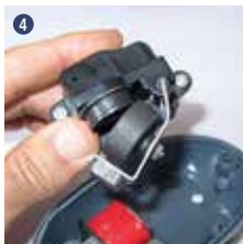
Removing the diaphragm from the air chamber
